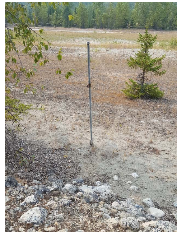
Photograph 36: North TSF, Cell 6, tailings surface and standpipe piezometer 6-3 (not functional), looking west. 8 August 2017.
