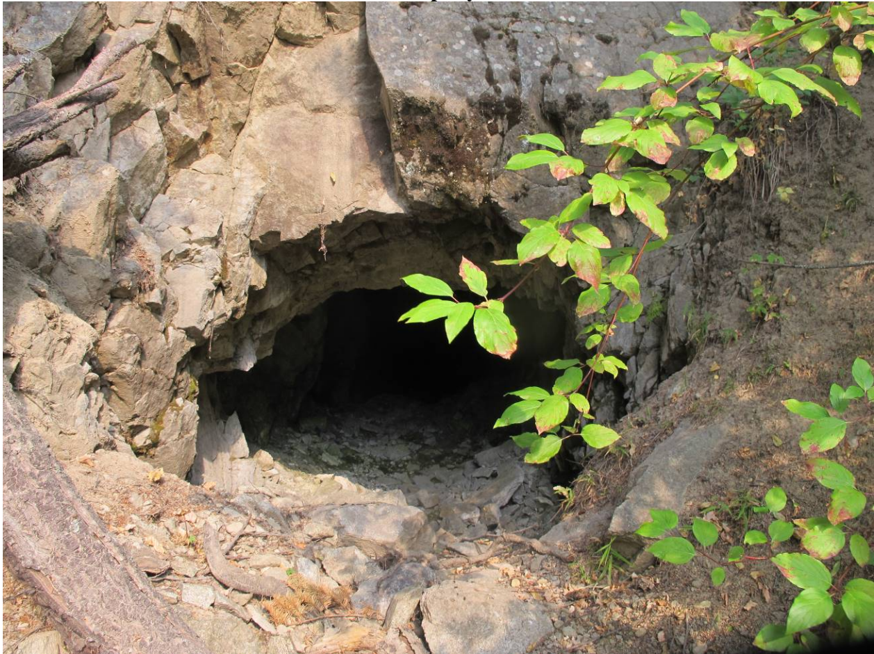
Photo 9: Abandoned adit providing access to underground workings outside of Beaverdell Mine Property
